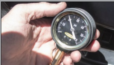
Large easy to read 2" dial gauge with 0-60 PSI operating range
